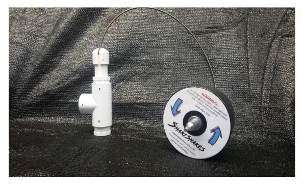
Once the cutting ball is started into the drain adapter, place the slotted 3/4" PVC cap around flexible shaft and push down onto the short piece of 3/4" PVC pipe.
